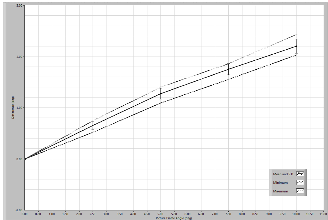
Figure 12. Difference of the average shear angle of the fabric, measured using laser scanner, and shear angle of the frame. Error bars indicate the standard deviation in five tests.
